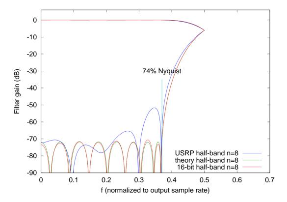
Finally, I can see that the author of the n=8 half-band filter incorporated in the USRP code base has not read this paper (since it wasn't written yet). The concept is sound, but the (non-zero) filter coefficients would better changed from [-16 74 -254 669 -1468 2960 -6158 20585] to [-49 165 -412 873 -1681 3135 -6282 20628].
