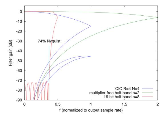
This figure above shows two other filters that use fewer multipliers than the full half-band filter. The fourth-order CIC filter (as used in the USRP) decimates by a factor of four, so more frequencies alias onto the pass band. This effect is shown by additional folding in its response curve. It is versatile, with its decimation ratio easily configured on-the-fly.
