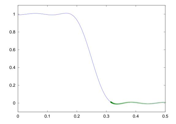
Properly refining the coefficients to make each ripple exactly the same size is a bothersome exercise, but one with a well established lore in curve-fitting circles. The final shape within the stop band (and, by symmetry, the pass band) is patterned after a Chebyshev polynomial of order 2n.
