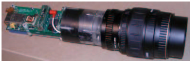
Figure 4: Camera assembly including CCD, acquisition, and networked computer
