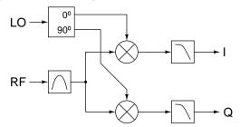
When the signal processing path is used in a feedback loop, choosing the output filter ends up as an awkward compromise between group delay and second harmonic rejection.
