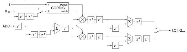
Manipulating the r and  $\theta$  inputs to the CORDIC allow this circuit to match gain and phase of multiple channel inputs to a vector sum. The output I, Q stream is thus ready to be summed across per-cavity instantiations.
